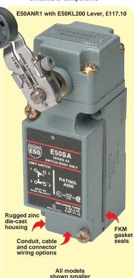
Ambient Temperature Range—Standard **Standard without Cable:** -10 to 121°C Standard with Cable: -10 to 105°C Low Temperature without Cable: -40 to 121°C Low Temperature with Cable: -40 to 105°C **Repeat Accuracy—Standard** Side Operated: Within 0.03 mm Top Operated: Within 0.008 mm Side Rotary: Within 0.04 mm **Torque Requirements:** Switch Body Screws: 29 to 35 Kg/cm Operating Head Screws: 16 to 21 Kg/cm
