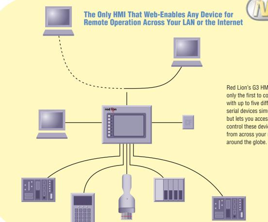
Red Lion's G3 HMI Series is not only the first to communicate with up to five different types of serial devices simultaneously, but lets you access, monitor and control these devices remotelyfrom across your network, or
