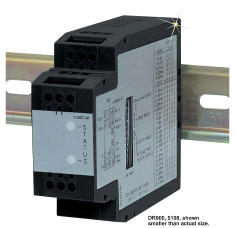
The modules' overall full scale accuracy typically exceeds 0.05% depending upon range selection and scaling. The microprocessor based design provides ease of field scaling and the onboard EEPROM stores scaling values for future recall. Both models come factory precalibrated for all input and output ranges. Factory or custom field scaling can be selected by a simple mode switch change.
