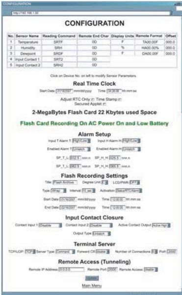
With the easy Web-based setup page, the two relays can be programmed for any combination of temperature or humidity, and high or low set points, as well as alarm conditions triggered by contact closures. The relays can also be programmed to turn off when conditions return to normal, or programmed to remain latched and require a manual reset.
