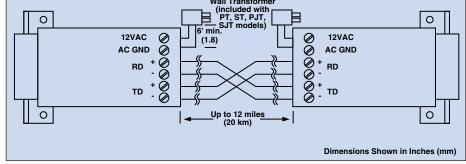
The LDM70 Series of products is designed to allow video display terminals (VDTs) and other RS-232 devices to be connected over distances sufficient to cover any industrial or institutional complex of buildings. These modems feature a rugged aluminum enclosure small enough to mount on the back panel of VDT units, saving valuable desk and floor space.
