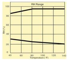
Relative Humidity Measurement Range vs. Temperature
