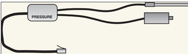
**Adaptor Type:** Complete with temperature and pressure sensors and connecting cable to logger
