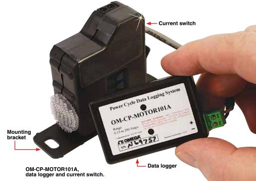
The OM-CP-MOTOR101A Series measures and records on and off status changes for motors or other equipment drawing up to 200 Amps. Simply route the current carrying wire for the equipment being monitored through the current switch. The state change occurs when the current switch exceeds the 150 mA set point. This allows for most basic equipment to be monitored. The current switch monitors whether there is current passing through a wire around which it is attached.
