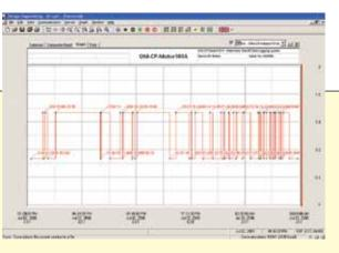
OM-CP-IFC200 Windows software displays data in graphical or tabular format, included with the OM-CP-MOTOR101A-KIT
