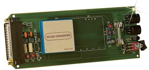
The OMB-DBK32A, \$649, shown smaller than actual size, provides additional power for OMB-LOGBOOK and OMB-DAQBOARD-2000 Series data acquisition systems
