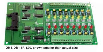
Outputs: 16 channels; TTL levels Output Low:
