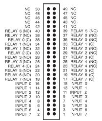
PCI-PDISO16 50-Pin Connector
