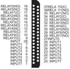
PCI-PDISO8 37-Pin Connector
