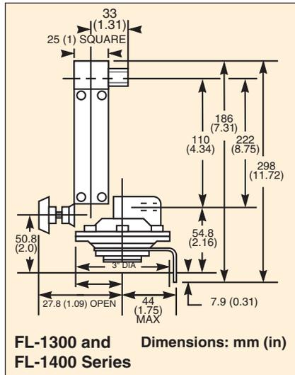
with correlation charts for air and water. The integral flow controller (for both the FL-1300 and FL-1400 Series) maintains a set flow rate when upstream line pressure varies.
