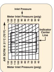
Convenient chart display allows user to correct for varying inlet pressures.
