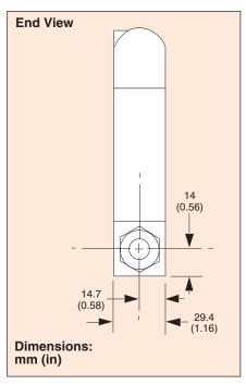
The FMA-5000 Series flowmeters measure molecular flow-the measurement of concern in most applications, including chemical processing, combustion, and heating or cooling. No temperature or pressure corrections are required, unlike with most other volumetric flow monitoring devices.
