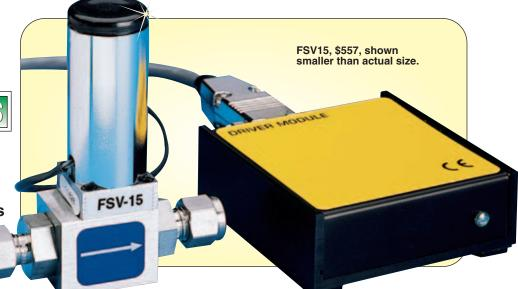
Driver Electronics: 7.62 W x 7.62 D x 25.4 mm H (3 x 3 x 1") Materials in Fluid Contact: 316 and 416 SS, FKM O-rings Maximum Pressure: 500 psig (3448 kPa) Maximum Differential Pressure: 50 psid (345 kPa); 35 psid (241 kPa) for FSV15 Leak Integrity: 1 x 10° sccs; helium, individually tested Ambient Temperature: 0 to 50°C (32 to 122°F) CE Compliance: EMC Directive 89/336/EEC EN55011:1991; Group 1,
