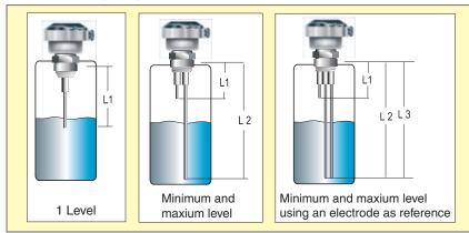
LVCP, shown smaller than actual size. LVCP switches are available with varying cable lengths to monitor and control different fluid levels. Cables may also be shortened by the user. Consult Flow Engineering for details.
