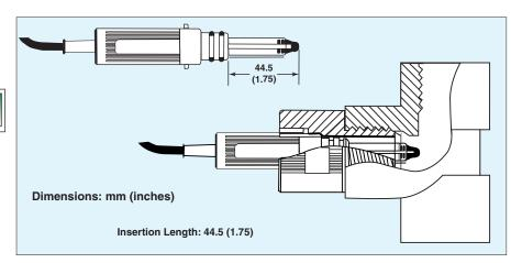
The PHE-5555-10 pH electrode allows for quick insertion using our simple "twist and lock" adaptor, as shown in the diagram above. This combination electrode incorporates pH, reference and solution ground in a robust PPS (Ryton®) housing. Double junction reference construction makes the PHE-5555 highly resistant to electrode poisoning.
