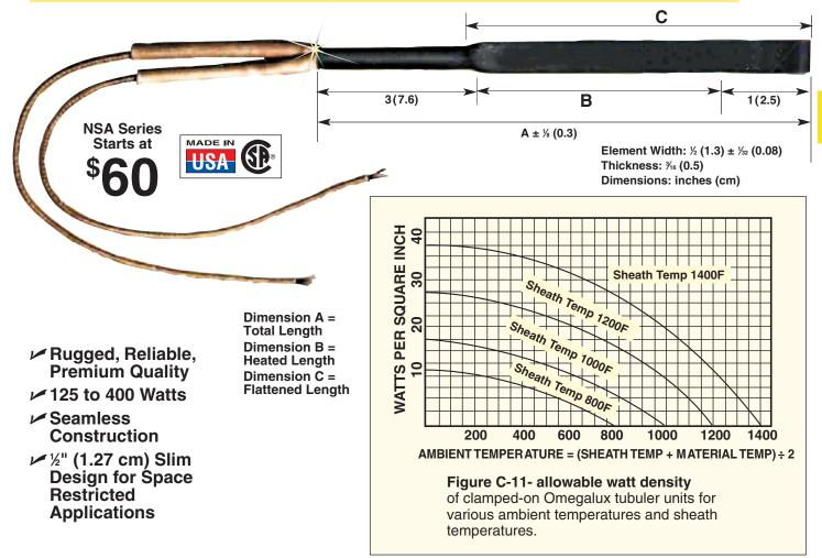
The NSA series high temperature strip heater features a slim ½" (1.27 cm) width design, ideal for heat applications where space is restricted. The maximum temperature rating is 260°C (1500°F) with Incoloy sheath material. Applications include heating of large tanks, vats and heating ducts while clamped to the surface.
