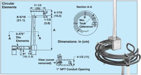
tank. These heaters are convenient answers for many immersion. Heating applications capacities, dimensions and sheaths fit a wide range of heating applications. Easy to install and remove for cleaning with straight or circular element designs to fit many tank configurations.
