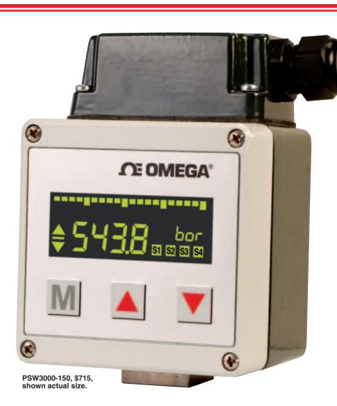
Power Supply: 18 to 32 Vdc, reversed polarity protected A/D Converter: Resolution: 12 bit (4096 steps per span) Scanning Rate: 1000/sec Time Constant: Approx 40 sec Analog Output Current Output: 4 to 20 mA **Load:** Max RI = 600  $\Omega$  at 24 Vdc excitation Load Influence:  $0.3\%/100 \Omega$ Scanning Rate: 1 msec Voltage Output: 0 to 10 Vdc Rating: Max 10 mA, short circuit-proof Adjustment Range: 25 to 100% FS
