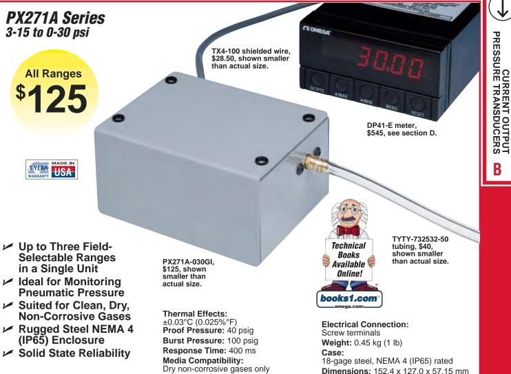
The OMEGA® PX271A pressure transducer is ideal for use in pneumatic control systems and other industrial applications. The sensing element is a 100% solid state piezoresistive silicon chip featuring low hysteresis, excellent repeatability, and long-term stability. The signal conditioning and temperature compensation are performed by industrial-quality integrated circuits to provide an accurate, linear, user-selectable 0 to 5 or 0 to 10 Vdc signal.
