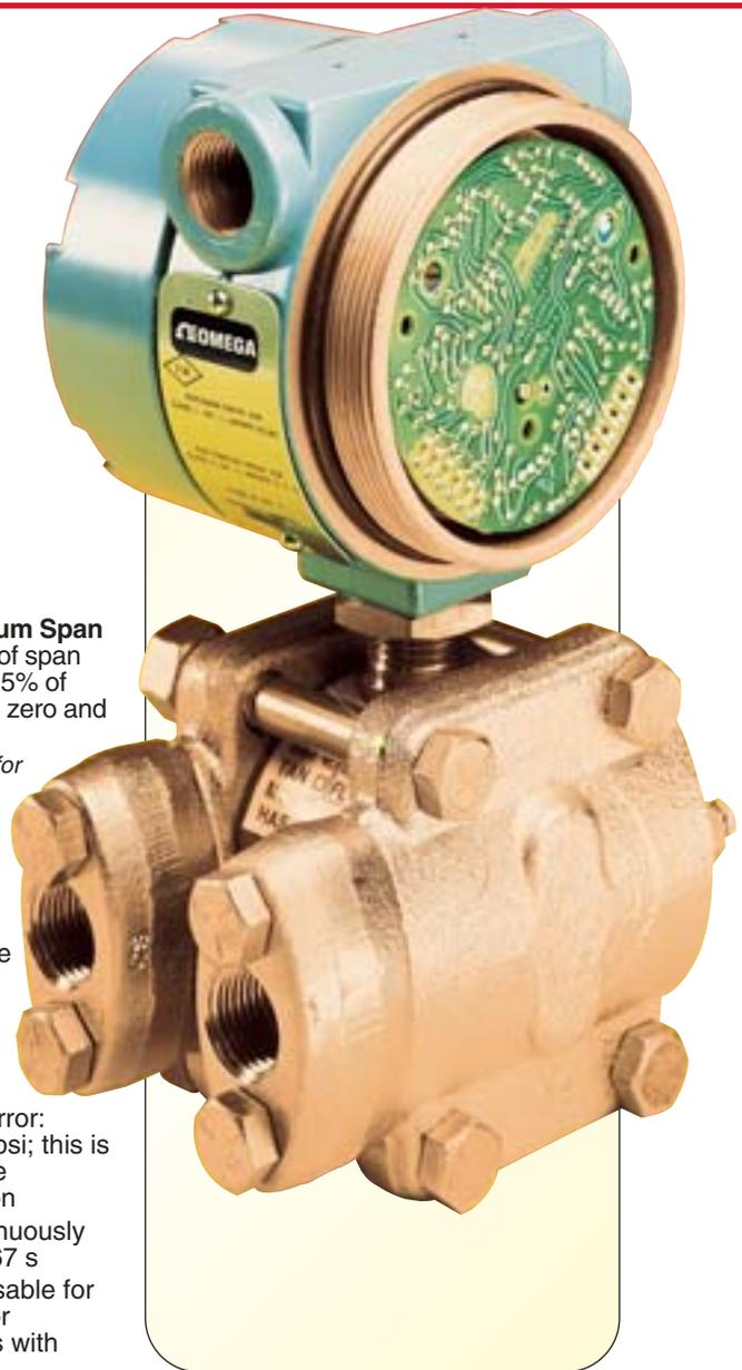
**Temperature Effect at Maximum Span 0 to 150 inH<sub>2</sub>O:** Zero error ±3% of span per 55°C (100°F); total error ± 3.5% of span per 55°C (100°F) (includes zero and span errors)
