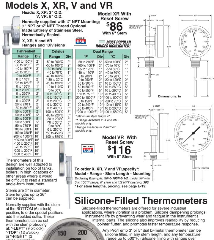
thermometers can be se with the stem protruding at: "-LEFT" (9 o'clock), "-TOP" (12 o'clock) or "-RIGHT" (3 o'clock) positions. If not specified, the standard BOTTOM (6 o'clock) position will be supplied.
