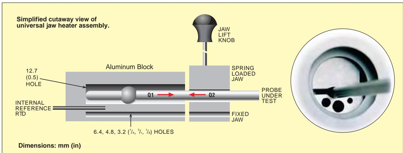
5-hole block diameters: 1.6, 3.2, 4.8, 6.4, and 9.5 mm (1/16, 1/8, 3/16, 1/4, and 3/8").
