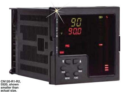
· During output "on", the control measures load current and generates an alarm condition when this current is lower than a pre-programmed threshold value (a low current shows a partial or total break down of the load or of the actuator)
