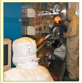
OMEGA's products making OMEGA's products. OMEGA uses Super OMEGACLAD® XL thermocouple probes in its Class 10 clean rooms to monitor critical process temperatures and achieve consistent, high-quality products.
