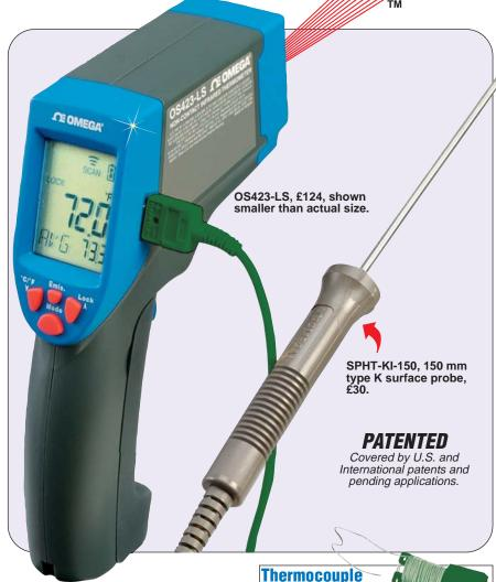
Emissivity Range: 0.95 default; adjustable 0.1 to 1 step 0.01 Resolution (-9.9 to 199.9°C):
