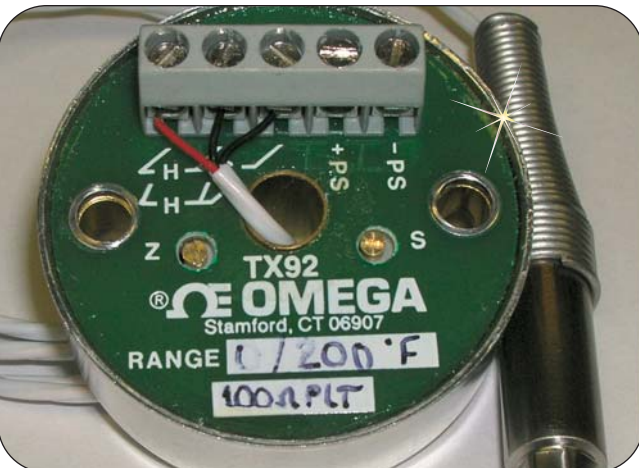
TX92 transmitter, £126, shown actual size (see omega.co.uk ).
