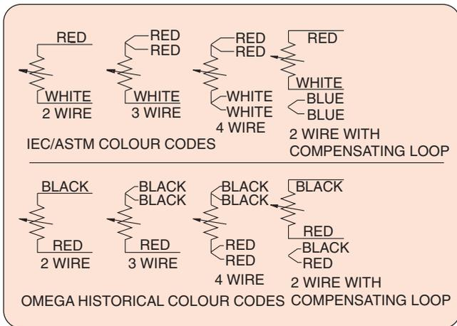
Except for the 2-wire configuration, each of the above wiring arrangements allows the monitoring or control equipment to factor out the unwanted lead wire resistance and other resistances that occur in the circuit.
