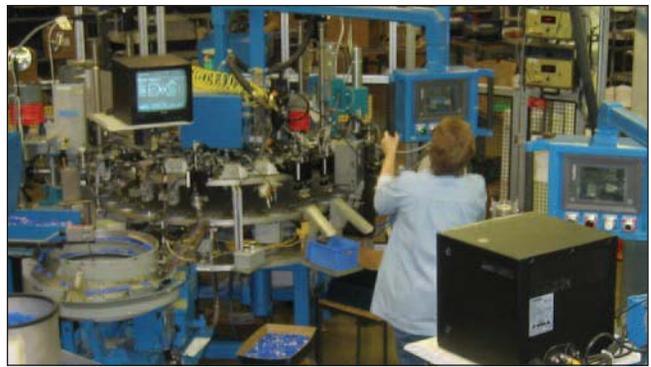
One of OMEGA's automated connector manufacturing lines
